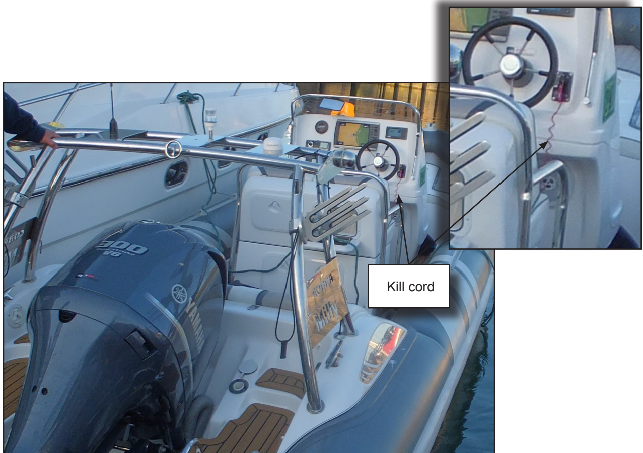
Figure 1: Boat with kill cord in place
